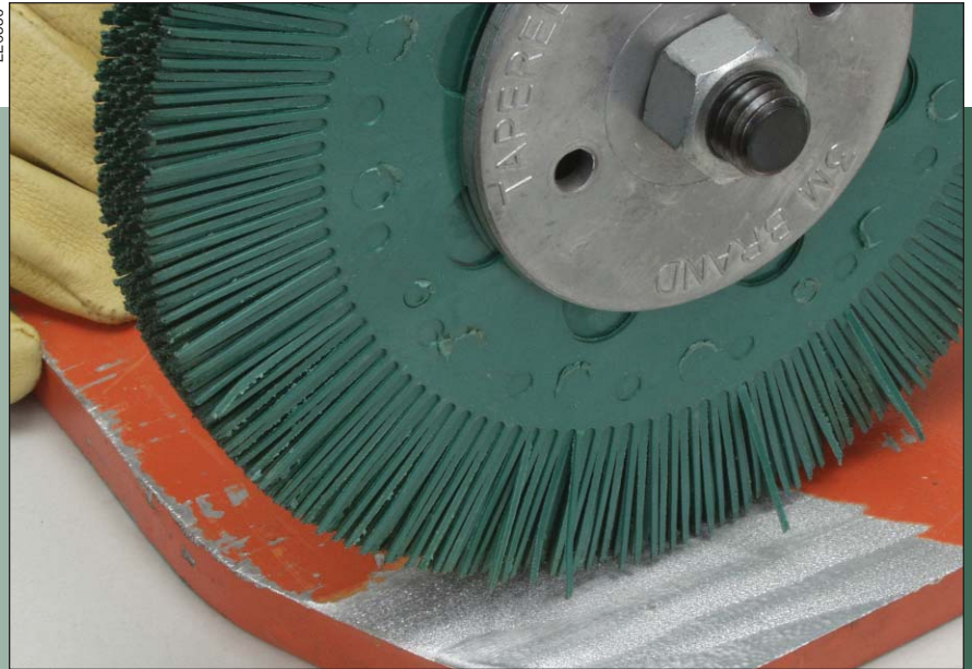
8" Radial Bristle Brush, grade 50, removing paint from straight shaft tool.
